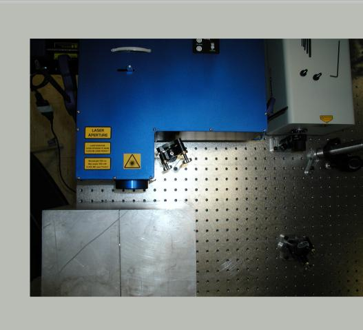
By focusing the beam of a pulsed Nd:YAG laser onto a small area of a sample, thermoelastic expansion in the sample results in broad-band ultrasonic wave propagation. A newly developed laser ultrasonic interferometer measures the absolute ultrasonic displacement for both the vertical and the radial component by collecting light scattered from the sample at high angles
