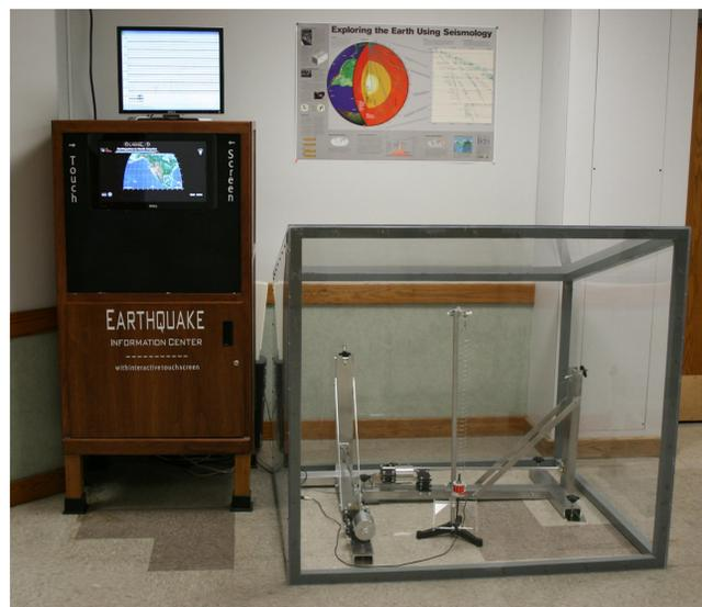
Boise State University's Seismic Station located on the main level of the Math & Geoscience building consists of three components - two horizontal Lehman's and a vertical Slinky seismometers. This is often the location of interviews with local media.
